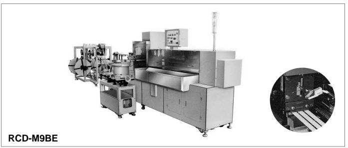
This automatic machine processes 2.0mm (0.79") and 2.5mm (.098") pitch jumper wires, including cutting to predetermined length, slotting, semi- or full-stripping and kinking. It also simultaneously fits insulation displacement connectors to one or both ends of the cable.
