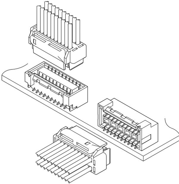
In order to correspond to the various high-density PC board designing, this GHD connector is designed as 1.25 mm pitch double row type connector. Provide a full lineup of 10 to 40 circuits for top and side entry types. Its operability is very well, in spite of the small size with tin-plated.
