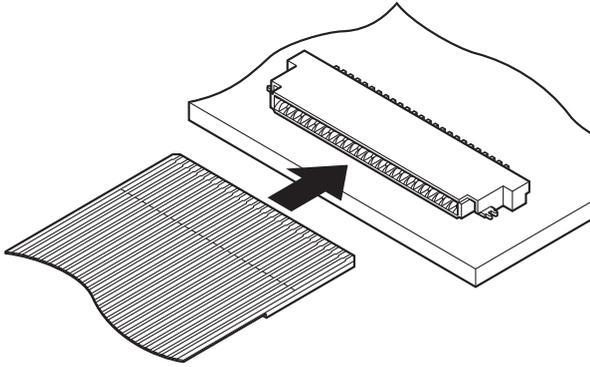
The large miniaturization at pitch direction and depth direction and low profile as 1.2 mm mounting height are realized. FH connector is miniaturized and space saving Non-ZIF type connector for FPC.
