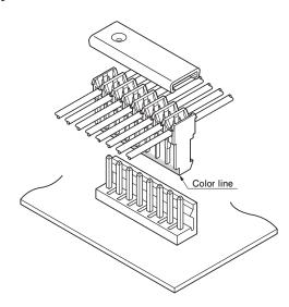
The VR series is a 3.96 mm pitch wire-toboard connector for 7 A rated power supply circuits. Furthermore, it can acccommodate AWG #18 wire, which is rare for an IDC connector.
