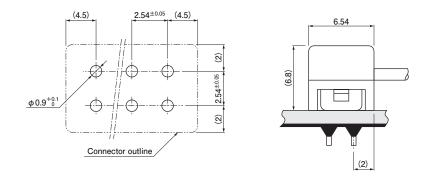
Note: 1. The figure of PC board layout is the figure viewed from the connector mounting side. 2. Tolerance for the PCB hole pitch shall be  $\pm$  0.05 and shall not accumulate.
