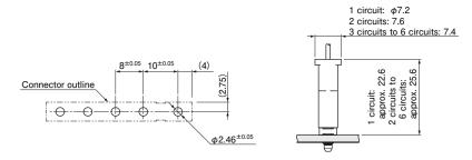
Note: 1. The figure of PC board layout is the figure viewed from the connector mounting side.
