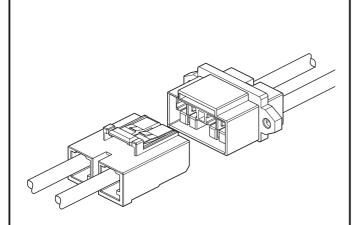
One-touch connection and disconnection connector corresponding to high current. This is a wire to wire connector, which current rating is 50 A capability in 2-circuit, and male and female contacts of this connector is designed as the same shape.
