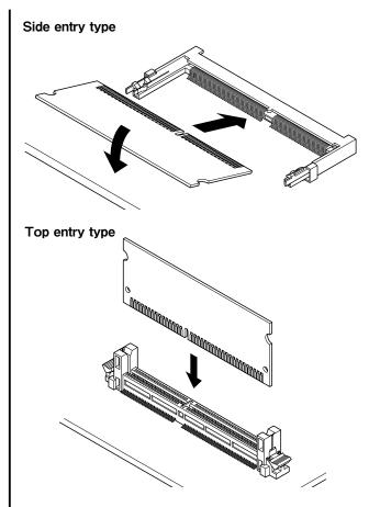
This is sockets for the S.O.DIMM of 144-circuits based on the JEDEC MO-190 standard, and its side type socket is low profile with 5.2 mm height.
